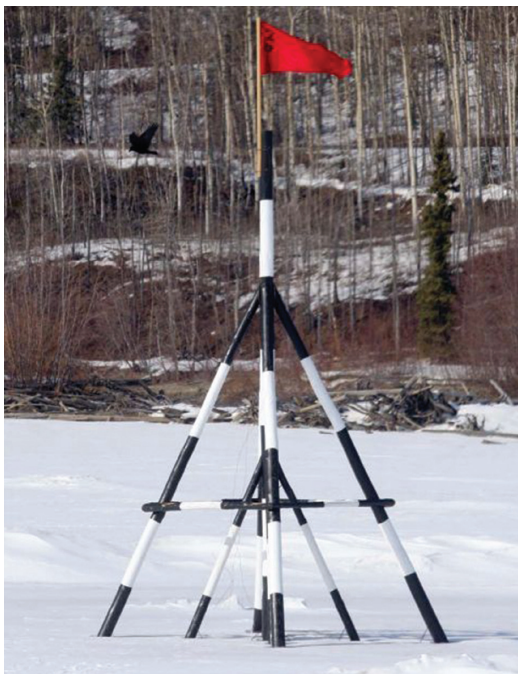
Each year, a town holds a contest to predict the exact time the ice will break on the river. People build a tripod like this Nenana Ice Classic tripod and set it on the ice. It connects to a clock inside a wooden tower on the dock. When the ice breaks, the tripod starts to move, trips a wire, and instantly stops the clock.
